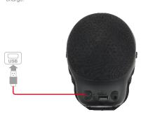
Connect the USB-A plug to a charger with a 5W power output, and insert the Micro USB plug into the charging port.
